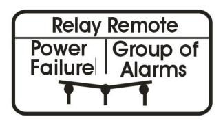
• When everything is ok, and when the device is switched on, both relay contacts are "short-circuited", if an alarm occurs, the relay contact "opens".
